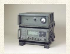
Datron's rugged, 400W mobile system is completely sealed and ideally suited for applications requiring use in harsh environments. The RT7000/RA400 system (shown above) can be used in either mobile or shipboard installations. It is rated for full continuous-duty operation.
